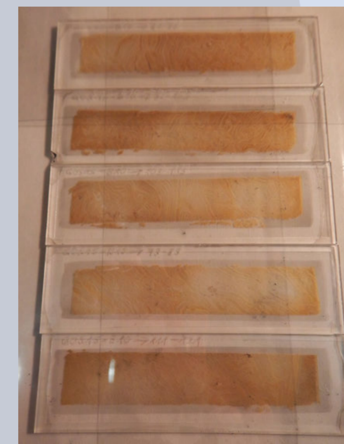
8. finished covered thin sections for microscopy – size 120 x 35 mm
