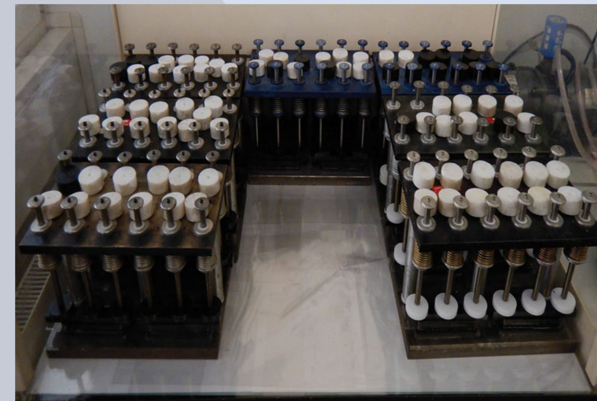
4. glued samples under pressure blocks
