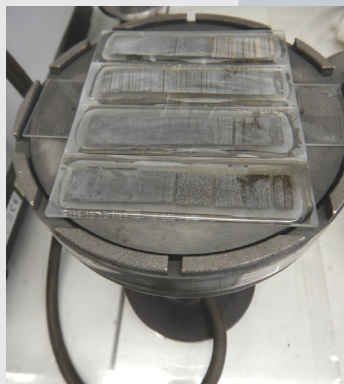
6. samples on Logitech vacuum head PLJ7
