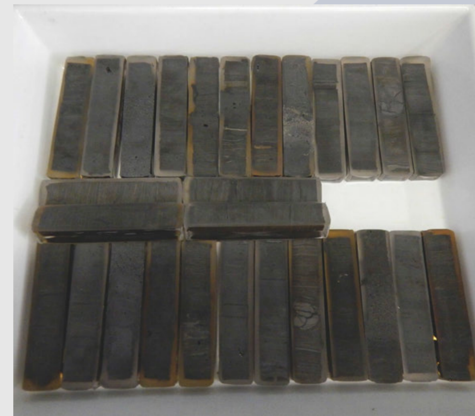
3. sediment blocks – impregnated and ground shallow
