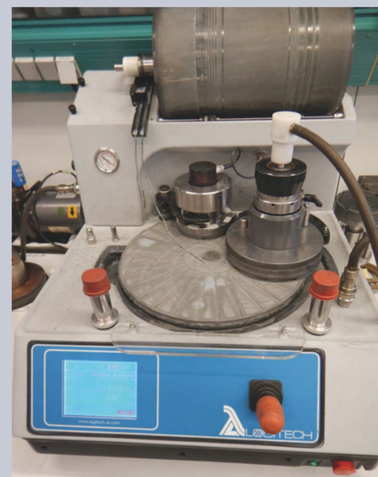
7. lapping the samples to finale size with Logitech LP50
