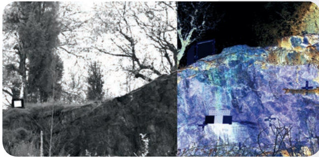
left: panchromatic VNIR outcrop scan right: principal component composite image showing the spectral variety of the material in the image scene
